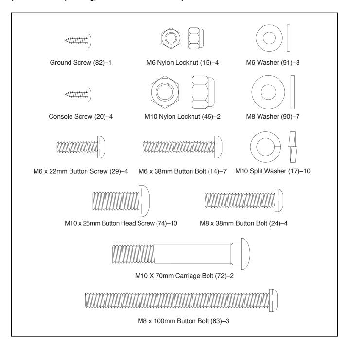
Attach the Front Stabilizer (2) to the front of the Frame (1) with two M10 x 70mm Carriage Bolts (72) and two M10 Nylon Locknuts (45). Make sure that the Front Stabilizer is turned so the Wheels (75) are not touching the floor.
